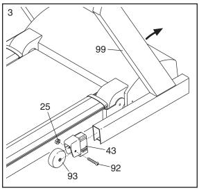
With the help of a second person, carefully lower the Uprights (99). Make sure that the Wheel Housings (43) remain in the bases of the Uprights.
